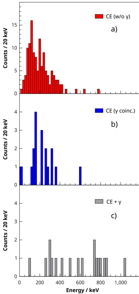
Figure 8: Energies of conversion electrons from the ER-CE-(CE)-SF/ $\alpha$  correlations. a) electrons not coincident with  $\gamma$  rays, b) electrons in coincidence with  $\gamma$  rays, c) summed energies of electrons and coincident  $\gamma$  rays.
