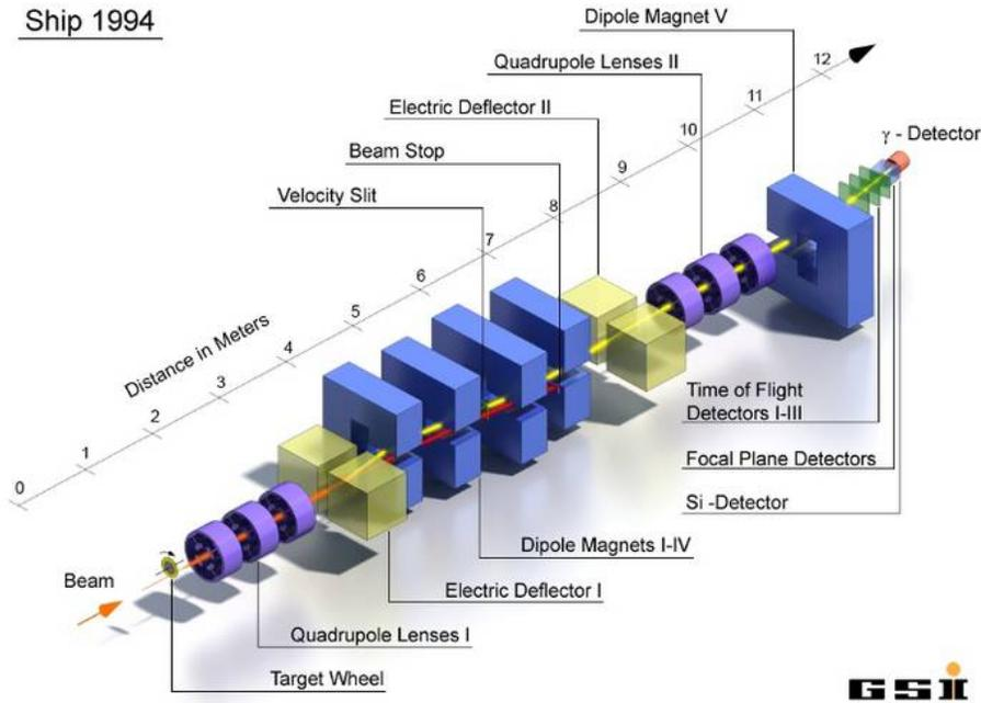
Figure 3: Velocity filter SHIP [24].
