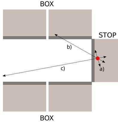
Figure 5: Schematic view (not to scale) of STOP and BOX detectors registering fragments from SF of an implanted nucleus (side view with respect to the direction of implantation). Red circle represents an evaporation residue implanted into the STOP detector, arrows represent the directions of 2 fission fragments. Active area of Si detectors is in bright grey color, dead layers are in dark grey. From the geometrical point of view, three possible cases can occur:
