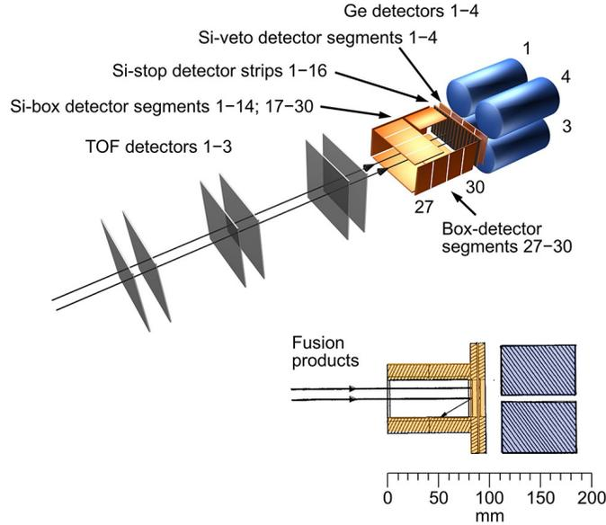
Figure 4: Detection system at velocity filter SHIP [26].
