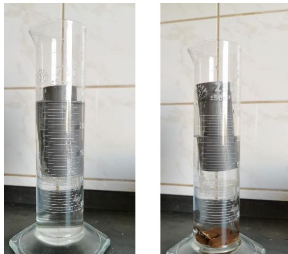
Figure 5. Left: The beginning of the demonstration. The coins are inside Archie while Archie is afloat. Right: The coins are in the water. The water level visibly drops.
